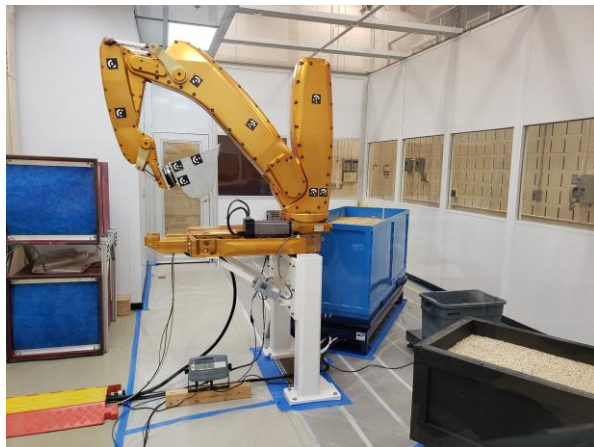
Fig. 1. - Excavation Lab at NASA Glenn Research Center houses the Advanced Planetary Excavator (APEX) and soil bins inside a dust enclosure.
